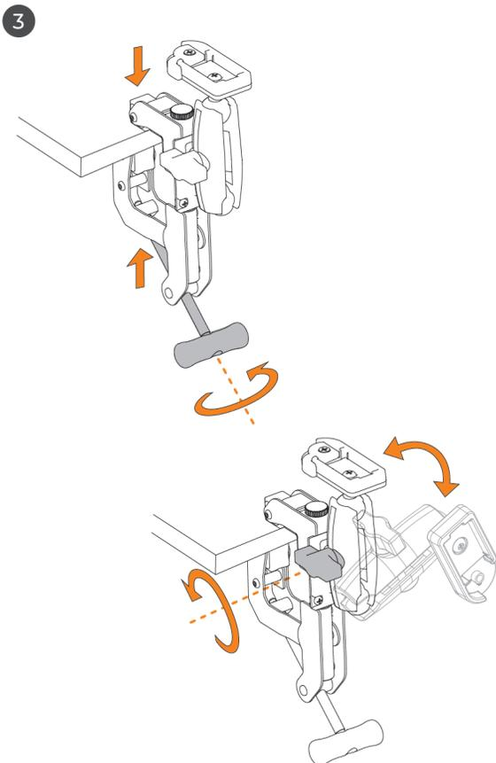
1. Attach Camera Clamp to a desired location, tightening the handle.
