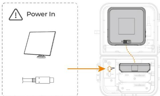
The BCC5000 waterproof power box has an additional battery expansion slot, which can be installed with up to 3 Brinno rechargeable battery packs (MRB1000), which will charge the TLC5000 camera.
