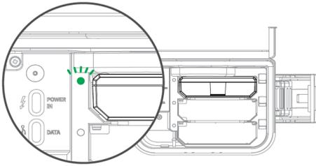
When the battery pack is inserted into the housing, the LED flashes to indicate the battery is connected.
