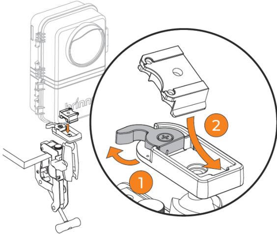
1. Loosen the locking switch.
